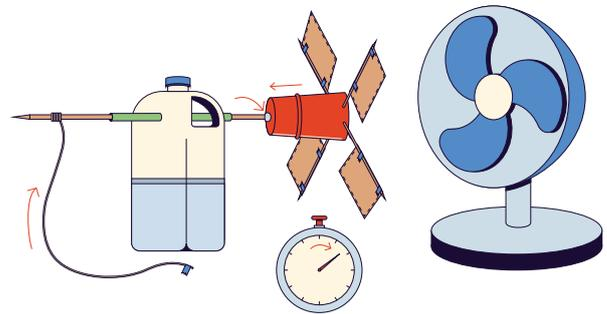
8. Attach a marked piece of string to the skewer and use the stopwatch to time how long it takes to wind that length of string around the skewer.
