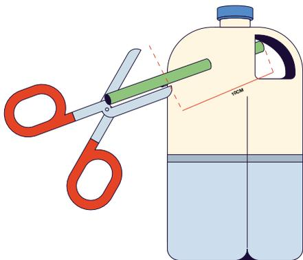
3. Push the straw through both of the small holes you cut into the bottle. Trim the ends of the straw so just a centimeter or two sticks out of each side.
