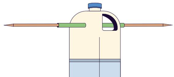
4. Insert the skewer into the straw. This is the base of the turbine ready to have blades mounted.
